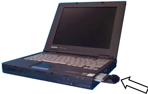
Figure 1 - Laptop Card Installation
