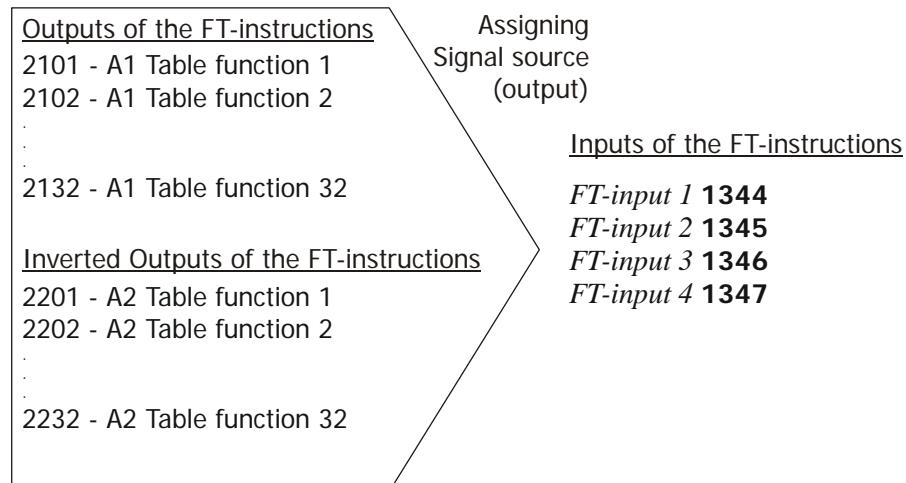
**Example of link of FT-instruction input to an FT-instruction output:** Output 1 of FT-instruction 2 (index 2 of function table) is required for linking to another logic function. The logic status of the output is to be present at input 2 of function 3 (Index 3 of logic table).
