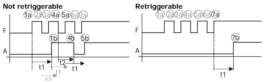
Processing like example 3. The positive edge 5a sets a high output. 6a and 7a follow in quick succession, so that these two edges are filtered out.
