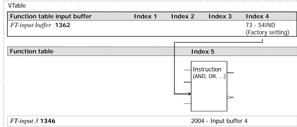
**2. Example:** Link of a FT-instruction input to a **signal source**: The signal "Warning Motor Temperature" is to be present at input 1 of function 2 (index 2 of table).
