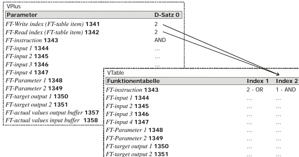
For parameterization using the function table VTable, the commissioning and diagnosis software VPlus, version 4 or higher is required.
