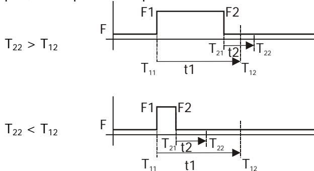
The delays are implemented as „retriggerable“ and „not retriggerable“ version.
