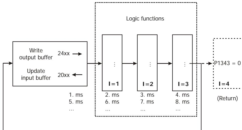
The function table is processed cyclically. In the first step, the output buffer is written to the global variables 24xx, and the input buffer is updated in sources 20xx. Then the FT-instructions are processed, starting with Index 1.
