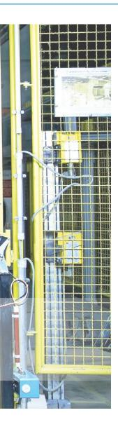
The deTec Ex II 3GD safety light curtains and the deTem Ex II 3GD multiple light beam safety devices from SICK meet the requirements of the ATEX guidelines for gas: II 3GD Ex nA op is IIB T4 GC X, and ATEX for dust: II 3GD Ex tc IIIB T135°C Dc. Both products provide maximum reliability and a very high level of safety for employees – even in explosive environments.
