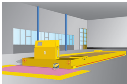
Lateral protection on an automated guided vehicle
