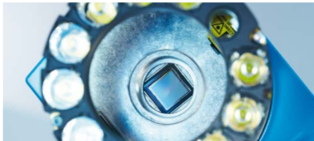
High-speed camera with a resolution of 2 or 4 megapixels and a dynamic focus for highly flexible reading performance
