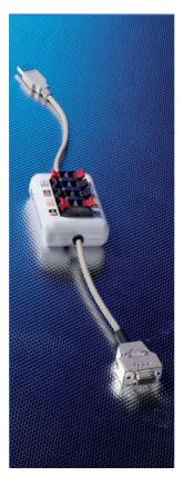
With the Programming Tool, every user, system integrator or distributor can self-configure any programmable version of the AFM/AFS60 via a PC or laptop. Resolutions up to 262,144 singleturn and 4,096 revolutions multiturn, zero point or offset and the counting direction can be freely selected.
