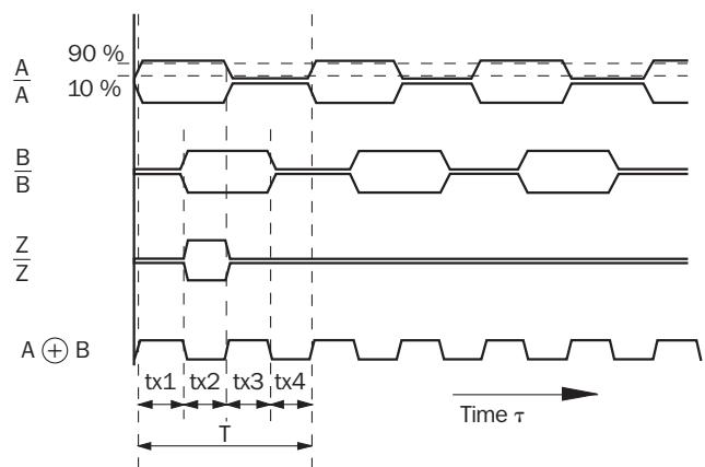
By linking the two signals A and B, an output signal is created whose cycle durations  $t_{x1} \dots t_{x4}$  have different sizes.
