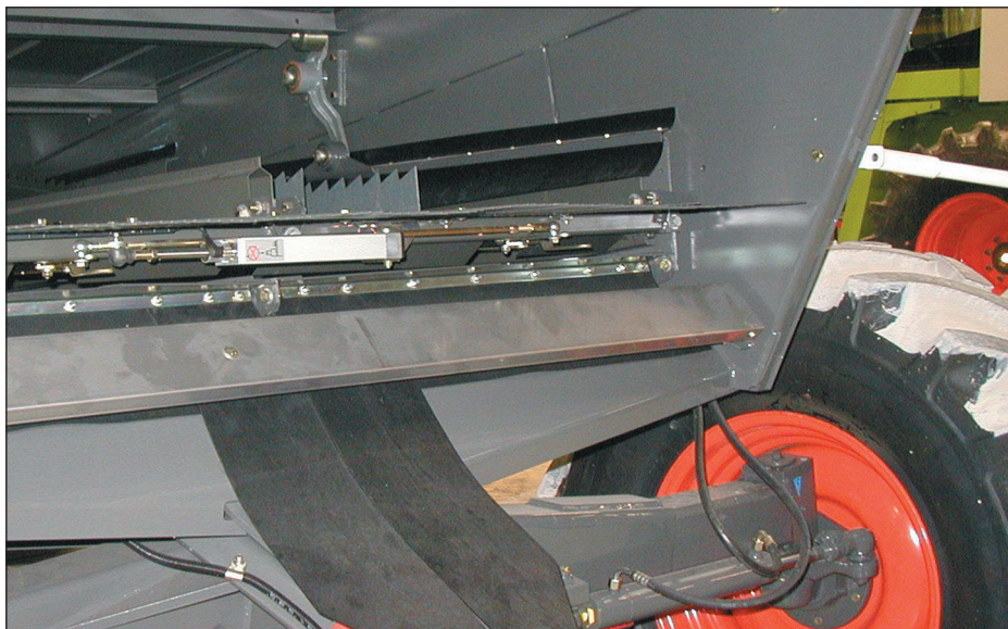
Adjustment of combine harvester sieve via series 010 electric cylinder. Ideal for use in harsh conditions (heat, dust and vibrations).
