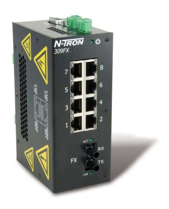
The switch has extended operating specifications to meet the harsh needs of the industrial environment, including extended temperature rating, extended shock and vibration specs, redundant power inputs, and a high MTBF (greater than 2M hours).
