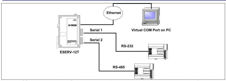
Virtual COM Mode - Allows a PC to communicate with serial devices through your network as if they were connected to a physical COM port on the PC.
