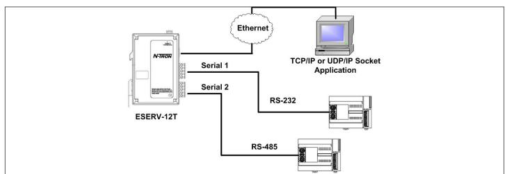
Direct IP Mode - Allows TCP/IP or UDP/IP socket applications to communicate directly with serial devices
