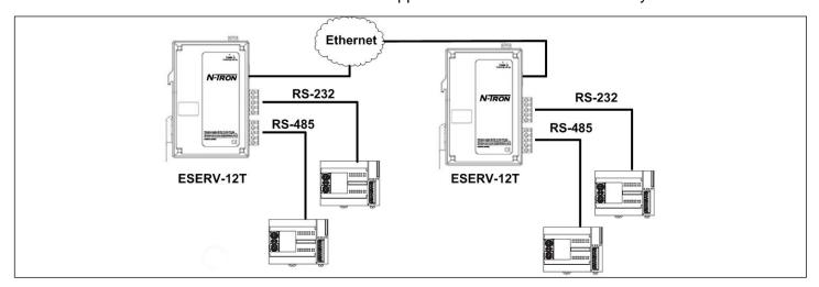
Paired Mode - Allows serial devices to communicate with each other by tunneling through your network.
