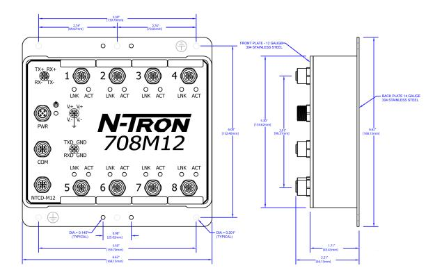
One (1) M12 A-Coded 5 Pin Female Port One (1) M12 A-Coded 5 Pin Female Port
