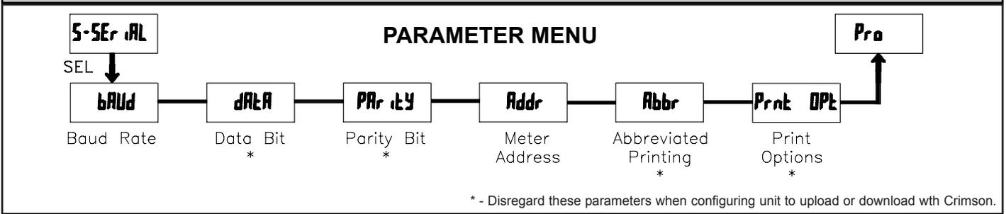
Module 5 is the programming module for the Serial Communications Parameters. The only parameters of concern when utilizing the CUB5USB programming option card to communicate with Crimson 2 programming software is the Baud Rate and Meter Address. The Parameters are only accessible when an optional CUB5USB, RS232 or RS485 serial communications card is installed in the meter.
