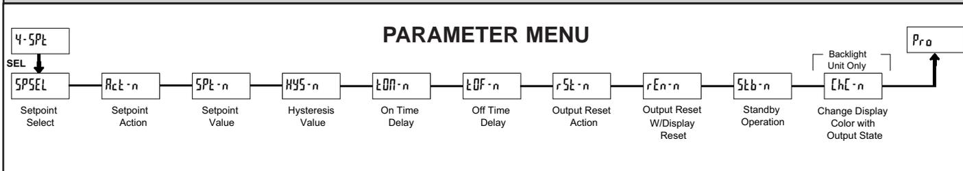
The Setpoint Output Parameters are only active when an optional output module is installed in the meter.
