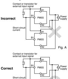
The PM5S series is provided with a transformer less power supply system.
