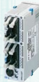
FPΣ (Sigma) Programmable Controller for sophisticated temperature control applications
