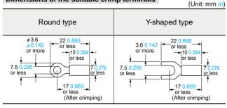
Note: Use crimp terminals with insulating sleeves.
