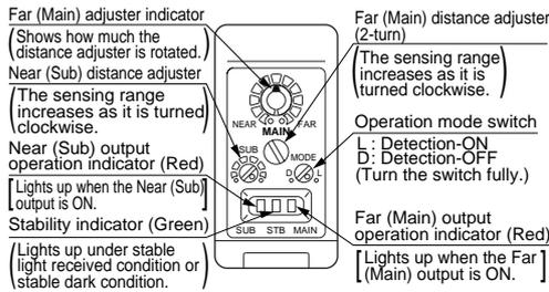
Notes: 1) Turn the distance adjuster gradually and lightly with the attached screwdriver.
