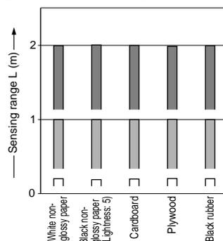
These bars indicate the sensing range with the respective objects when the distance adjuster is set at the sensing range of 2m, 1m and 0.2m long, each, with white non-glossy paper.
