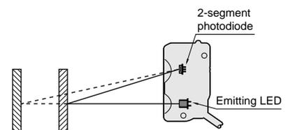
Sensing is based on the difference in the incident beam angle of the dotted line and the solid line in the above figure.
