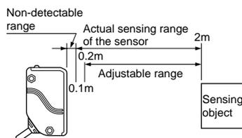
2) The Near (Sub) distance adjustable range, L<sub>2</sub>, changes with the setting of the Far (Main) distance, L<sub>1</sub>, as shown in the table below.
