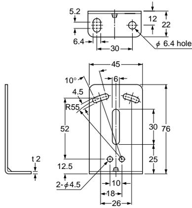
Material: Cold rolled carbon steel (SPCC)
