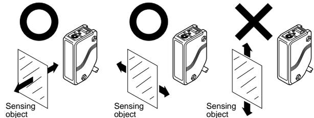
Do not make the sensor detect an object in this direction because it may cause unstable operation.
