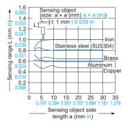
As the sensing object size becomes smaller than the standard size (iron sheet 5.4 × 5.4 × t 1 mm 0.213 × 0.213 × t 0.039 in), the sensing range shortens as shown in the left figure.
