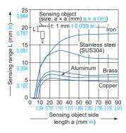
As the sensing object size becomes smaller than the standard size (iron sheet 54 × 54 × t 1 mm 2.126 × 2.126 × t 0.039 in), the sensing range shortens as shown in the left figure.
