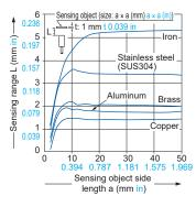
As the sensing object size becomes smaller than the standard size (iron sheet 15 × 15 × t 1 mm 0.591 × 0.591 × t 0.039 in), the sensing range shortens as shown in the left figure.
