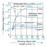
As the sensing object size becomes smaller than the standard size (iron sheet 12 × 12 × t 1 mm 0.472 × 0.472 × t 0.039 in), the sensing range shortens as shown in the left figure.
