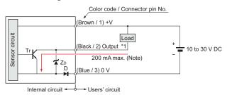
Note: In the case of the M8 threaded type: 200 mA max. (at -40 to +70 °C -40 to +158 °F), 100 mA max. (at +70 to +85 °C +158 to +185 °F)
