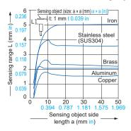
As the sensing object size becomes smaller than the standard size (iron sheet 18 × 18 × t 1 mm 0.709 × 0.709 × t 0.039 in), the sensing range shortens as shown in the left figure.
