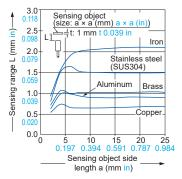
As the sensing object size becomes smaller than the standard size (iron sheet 8 × 8 × t 1 mm 0.315 × 0.315 × t 0.039 in), the sensing range shortens as shown in the left figure.
