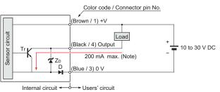
Note: In the case of the M8 threaded type: 200 mA max. (at -40 to +70  $^{\circ}$ C -40 to +158  $^{\circ}$ F), 100 mA max. (at +70 to +85  $^{\circ}$ C +158 to +185  $^{\circ}$ F)
