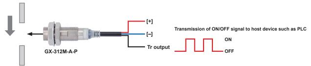
◆ When IO-Link compatible sensors are connected to the IO-Link master, they can transmit not only ON/OFF signal but also sensor level information and operation mode switching information in both ways. So, the sensors can be utilized for the visualization of manufacturing operations or for the incorporation of IoT technology.
