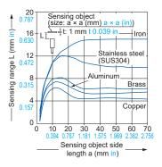
As the sensing object size becomes smaller than the standard size (iron sheet 45 × 45 × t 1 mm 1.772 × 1.772 × t 0.039 in), the sensing range shortens as shown in the left figure.
