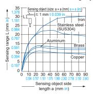
As the sensing object size becomes smaller than the standard size (iron sheet 90 × 90 × t 1 mm 3.543 × 3.543 × t 0.039 in), the sensing range shortens as shown in the left figure.
