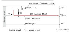
Notes: 1) In the case of the M8 threaded type: 200 mA max. (at -40 to +70 °C -40 to +158 °F), 100 mA max. (at +70 to +85 °C +158 to +185 °F)
