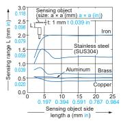
As the sensing object size becomes smaller than the standard size (iron sheet 8 × 8 × t 1 mm 0.315 × 0.315 × t 0.039 in), the sensing range shortens as shown in the left
