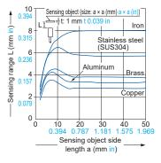
As the sensing object size becomes smaller than the standard size (iron sheet 24 × 24 × t 1 mm 0.945 × 0.945 × t 0.039 in), the sensing range shortens as shown in the left figure.
