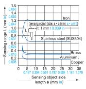
As the sensing object size becomes smaller than the standard size (iron sheet 4 × 4 × t 1 mm 0.157 × 0.157 in × t 0.039 in), the sensing range shortens as shown in the left figure.
