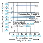
As the sensing object size becomes smaller than the standard size (iron sheet 3 × 3 × t 1 mm 0.118 × 0.118 × t 0.039 in), the sensing range shortens as shown in the left figure.
