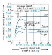
As the sensing object size becomes smaller than the standard size (iron sheet 12 × 12 × t 1 mm 0.472 × 0.472 × t 0.039 in), the sensing range shortens as shown in the left figure.
