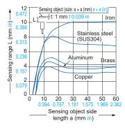
As the sensing object size becomes smaller than the standard size (iron sheet 30 × 30 × t 1 mm 1.181 × 1.181 × t 0.039 in), the sensing range shortens as shown in the left figure.
