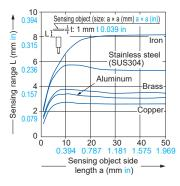
As the sensing object size becomes smaller than the standard size (iron sheet 24 × 24 × t 1 mm 0.945 × 0.945 × t 0.039 in), the sensing range shortens as shown in the left figure.
