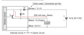
Note: In the case of the M8 threaded type: 200 mA max. (at -40 to +70 °C -40 to +158 °F), 100 mA max. (at +70 to +85 °C +158 to +185 °F)
