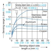
As the sensing object size becomes smaller than the standard size (iron sheet 48 × 48 × t 1 mm 1.890 × 1.890 × t 0.039 in), the sensing range shortens as shown in the left figure.
