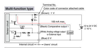
Symbols ... D<sub>1</sub>, D<sub>2</sub> : Reverse supply polarity protection diode Z<sub>D1</sub>: Surge absorption zener diode T<sub>r1</sub> : PNP output transistor T<sub>r2</sub> : NPN input transistor
