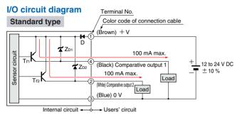
Symbols ... D : Reverse supply polarity protection diode ZD1, ZD2: Surge absorption zener diode Tr1, Tr2 : PNP output transistor
