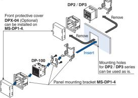
• An conversion bushing is available for when using the **DP-10**—**M** short pressure port type. It can be used to switch between this model and the **DP2 / DP3** series. When connecting to the pressure port, use a tightening torque of 1.0 N⋅m or less.
