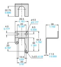
Material: Cold rolled carbon steel (SPCC)
