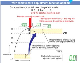
When remote zero-adjustment input is applied, the reference pressure is forced to "0". If the reference pressure changes to "20" or "40", the remote zero-adjustment input adjusts the reference pressure to "0" every time the reference pressure changes, so any variation in the filling pressure can be ignored.
