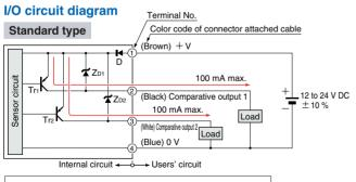
$Symbols \dots D: Reverse \ supply \ polarity \ protection \ diode \\ Z_{D1}, Z_{D2}: Surge \ absorption \ zener \ diode \\ T_{r1}, T_{r2}: PNP \ output \ transistor$
