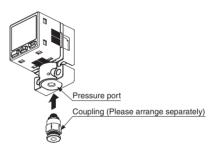
• When connecting the coupling to the pressure port of MS-DP1-FR/FE/FN, hold the pressure port with a 14 mm 0.551 in spanner and make sure that the tightening torque is 9.8 N⋅m or less
