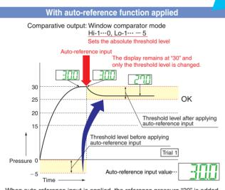
When auto-reference input is applied, the reference pressure "30" is added to the threshold level. If the reference pressure changes to "20" or "40", the auto-reference input compensates for this every time by changing the threshold level, so any variation in the filling pressure can be ignored.
