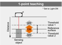
This method performs one-point teaching for the distance to the reference surface of the sensing object and sets the value obtained by subtracting the amount of shift from the result in threshold value 1 and the value obtained by adding the amount of shift to the result in threshold value 2.
