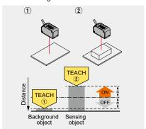
The threshold value is set automatically at the midpoint between the two points specified by teaching.
