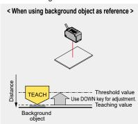
When the sensing object is located closer to the sensor than the background object, the threshold value for detection is set.
