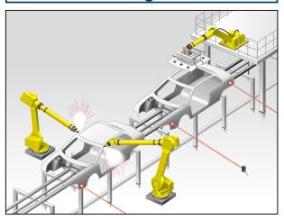
The long-distance sensing capability enables the installation of sensors at positions where they do not interfere with human workers or robot arm operation or at distant locations where the sensors will not be affected by scattering debris.
