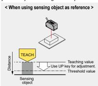
The threshold value is set on the background object side with reference to the sensing object. Use this method when there is a long distance to the background object.
