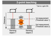
This method performs two-point teaching (sensing objects 1 and 2) for the two reference surfaces and sets the results in threshold value 1 and threshold value 2.
