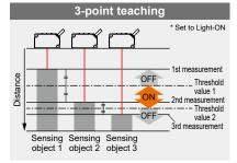
This method performs three-point teaching (sensing objects 1, 2 and 3) for the three references surfaces and sorts the teaching results in the descending order (Max, Middle, Min). Then, it sets the intermediate value between Min and Middle in threshold value 1 and sets the intermediate value between Middle and Max in threshold value 2.
