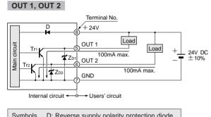
Symbols ... D: Reverse supply polarity protection diode ZD1, ZD2: Surge absorption zener diode Tr1, Tr2 : NPN output transistor
