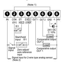
Notes: 1) COM. (0V) is internally connected to GND.2) If the shield wire of the analog sensor is connected, make sure to connect it to GND (Terminal No.7).
