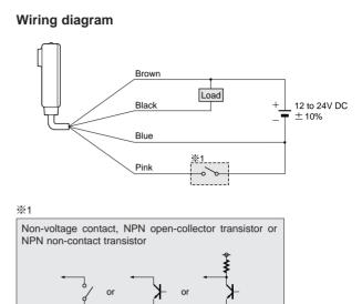
Low (-0.5 to +1.5V, or connected to 0V): sound-received-ON High (6V to supply voltage, or open): sound-blocked-ON
