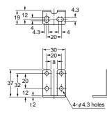
Material: Cold rolled carbon steel (SPCC) Two M4 (length 15mm) screws with washers are attached.
