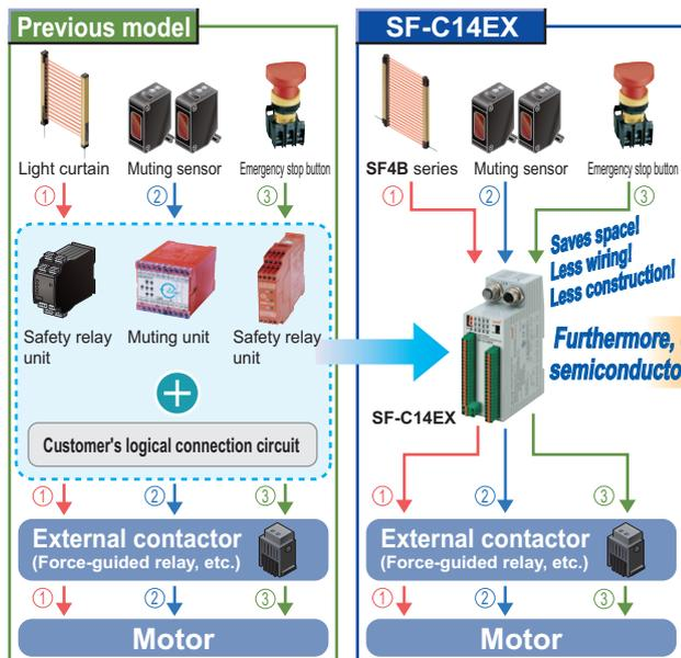
① Light curtain output circuit    ② Muting control circuit    ③ Emergency stop circuit
