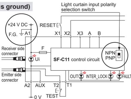
**Wiring diagram of SF-C12 and SF4B series (Control category 4)**
