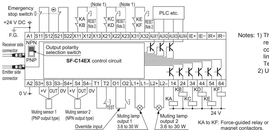
Notes: 1) The left diagram is when using manual reset. If automatic reset is used, disconnect the lead from X12 and X22, and connect them to X13 and X23 as shown by the dotted lines. In this case, a reset (RESET) button is not needed. Terminals X31 to X32 are for manual reset only.
