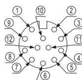
Note: Input and output for pin Nos. ⑩ and ⑫ are not used by this product
