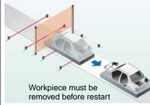
Removal operation required
