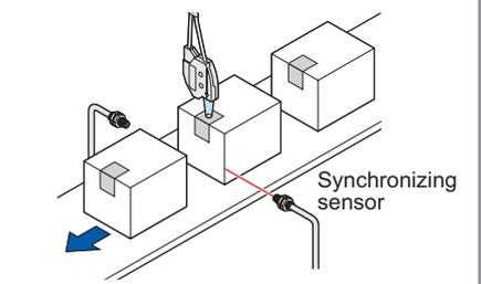
Notes: 1) **FD-L52** fiber head (high precision type) or **FD-L53** fiber head (extremely small spot type) is recommended for applications in which specular objects, having a high reflective index are to be detected, e.g., evaluating if metal objects are plated or not.
