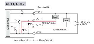
Symbols ... D: Reverse supply polarity protection diode ZD1, ZD2: Surge absorption zener diode Tr1, Tr2: NPN output transistor
