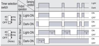
Delay time T: 10 ms approx. (when set to 10 ms), 40 ms approx. (when set to 40 ms)
