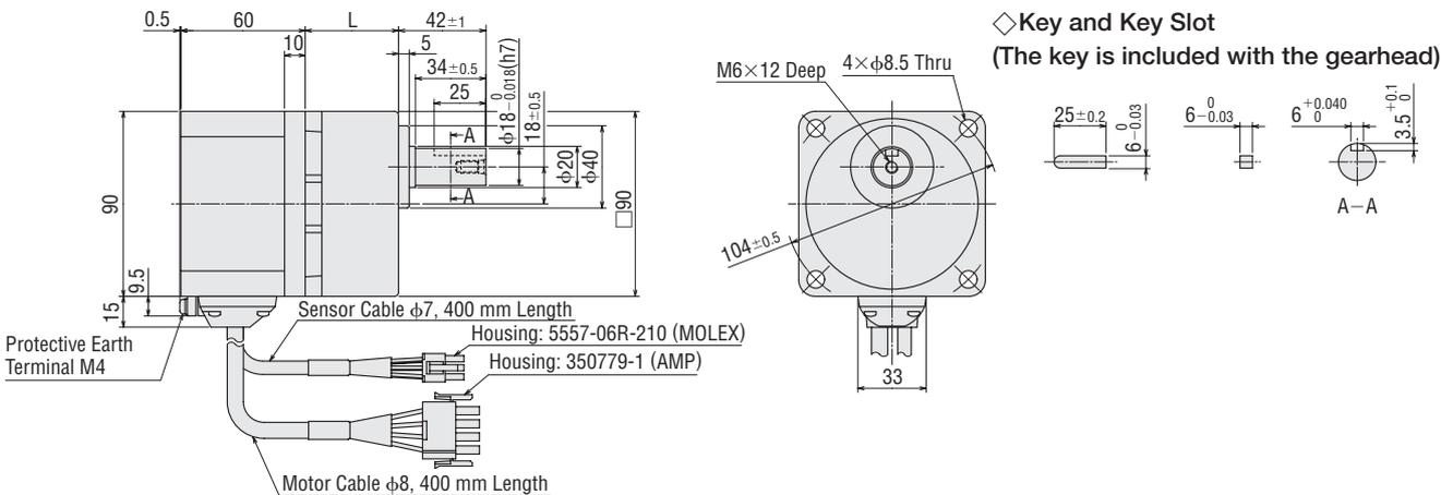
◇ Motor/Hollow Shaft Flat Gearhead
