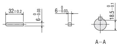
● At the time of shipment, a parallel key is inserted on the gearhead's shaft.
