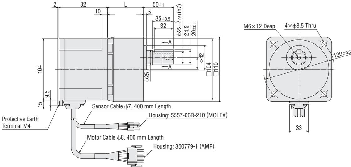
◇ Key and Key Slot (The key is included with the gearhead)
