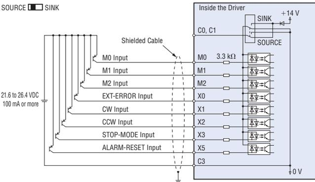
Controlled by Transistor
