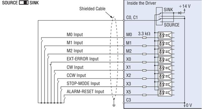
Controlled by Transistor
