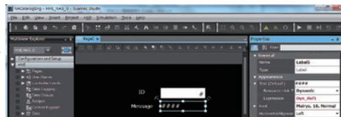
Set a variable for the ID to switch the group in the properties.
