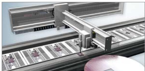
The chip molding process is another candidate application. In this case the actual chip must be placed in high speed, but also very accurate.
