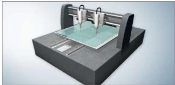
This glass cutting machine has high demands on continues and smooth movement as each misalignment is directly visible. The Sigma-5 servo in combination with the Trajexia motion control give full control of each movement.
