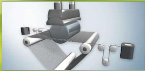
Flow wrap machine require various servo axes working in absolute synchronisation. Sigma-5 in combination with Trajexia allows synchronisation over the field proven Mechatrolink bus., greatly simplifying system wiring and reducing the chance on wiring errors.
