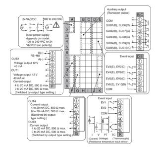
Note The power supply voltage must be 100 to 240 VAC or 24 VAC/DC for the E5AR-T to comply with CE marking requirements. The power supply voltage must be 100 to 120 VAC or 24 VAC/DC for the E5AR-T to comply with UL requirements.
