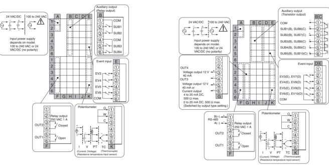
Note The power supply voltage must be 100 to 240 VAC or 24 VAC/DC for the E5AR-T to comply with CE marking requirements. The power supply voltage must be 100 to 120 VAC or 24 VAC/DC for the E5AR-T to comply with UL requirements.
