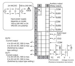
**Note** Note The power supply voltage must be 100 to 240 VAC or 24 VAC/DC for the E5ER-T to comply with CE marking requirements. The power supply voltage must be 100 to 120 VAC or 24 VAC/DC for the E5ER-T to comply with UL requirements.
