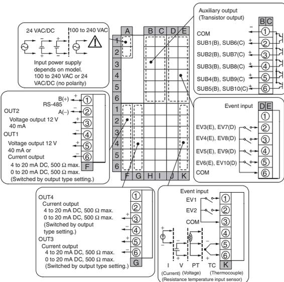
**Note** The power supply voltage must be 100 to 240 VAC or 24 VAC/DC for the E5AR-T to comply with CE marking requirements.
