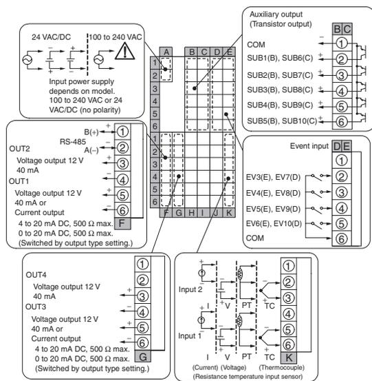
**Note** The power supply voltage must be 100 to 240 VAC or 24 VAC/DC for the E5AR-T to comply with CE marking requirements. The power supply voltage must be 100 to 120 VAC or 24 VAC/DC for the E5AR-T to comply with UL requirements.
