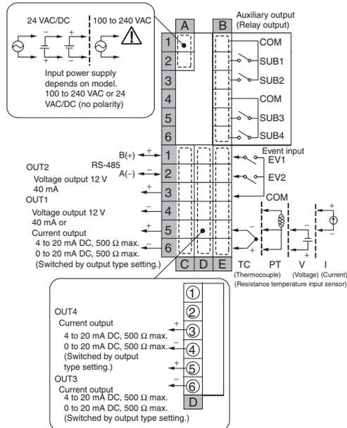
**Note** The power supply voltage must be 100 to 240 VAC or 24 VAC/DC for the E5ER-T to comply with CE marking requirements.
