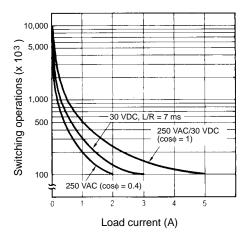
Reference: A maximum current of 0.15 A can be switched at 125 VDC (cosφ = 1) and a maximum current of 0.1 A can be switched if L/R is 7 ms. In both cases, a life of 100,000 operations can be expected.
