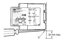
The H3DR can be mounted and dismounted with ease if a distance of 30 mm or more is kept between the H3DR and other equipment.
