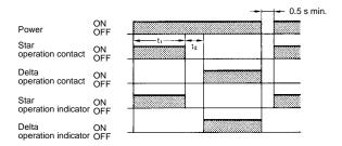
Note: t<sub>1</sub>: Star operation time setting t<sub>2</sub>: Star-delta transfer time
