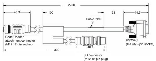
Note: Connect V430-W8 to I/O connector (M12 12-pin plug) and connect to a power supply.
