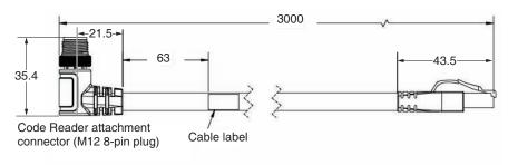
Cordset, M12 8-Pin Plug to RJ45 Ethernet 5 m Straight V430-WE-5M
