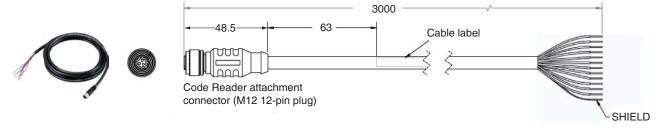
Cordset, M12 12-Pin Socket to Flying Leads 3 m Right angle down V430-W8LD-3M
