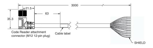
Cordset, M12 12-Pin Socket to Flying Leads 5 m Straight V430-W8-5M
