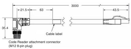
Cordset, M12 8-Pin Plug to RJ45 Ethernet 3 m Right angle up V430-WELU-3M
