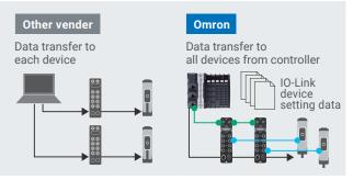
Configuring all devices at once from the controller eliminates the need to configure each device individually, greatly cutting down setup time.
