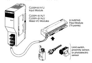
Note: B7A-series high-speed models cannot be used with C200H-B7AI1 and C200H-B7AO1.
