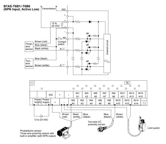
Note: 1. IEC wire colors for photoelectric sensors and proximity sensors are shown first. The colors in parentheses refer to the old colors.
