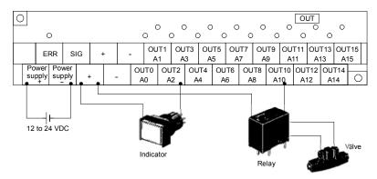
Note: Do not short-circuit terminals  $A \square \square$  and  $B \square \square$ , otherwise the internal element(s) of the B7A may be damaged.
