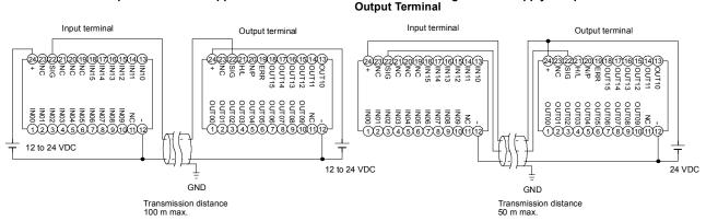
Note: A shielded cable with a thickness of 0.75 mm<sup>2</sup> min. must be used for signal transmission. It is recommended that the shield be grounded.
