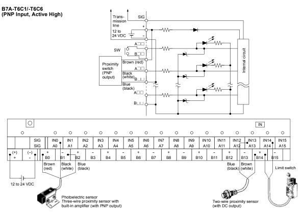
Note: 1. IEC wire colors for photoelectric sensors and proximity sensors are shown first. The colors in parentheses refer to the old colors.
