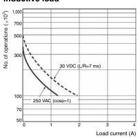
A current of 0.15 A max. can be switched at 125 VDC ( $cos\phi=1$ ) and current of 0.1 A max. can be switched if L/R=7 ms. In both cases, a life of 100,000 operations can be expected.
