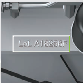
Presence inspection of marked characters
