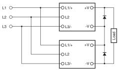
Note: 1. If the load is short-circuited, a reverse voltage will be generated inside the Power Supply. If this occurs the product may possibly deteriorate or be damaged. Always connect a diode as shown in the figure. Select diodes with the following ratings.
