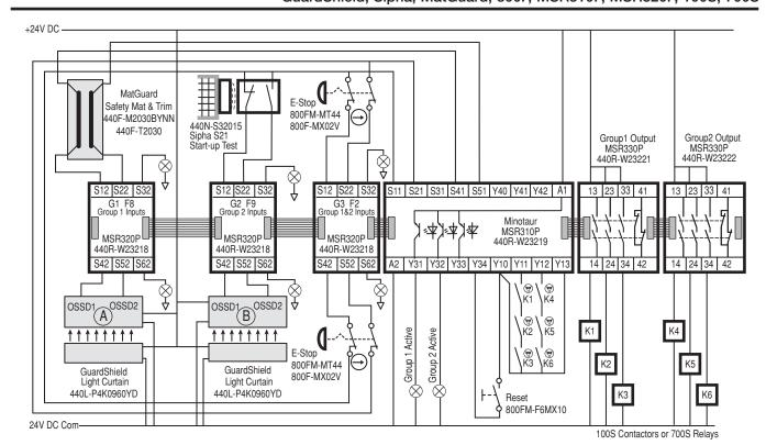
The light curtains are unobstructed. The safety gate is closed. The e-stops are reset, and the safety mat is unoccupied. The MSR330P outputs are off. K1-K6 are ready to be energized.
