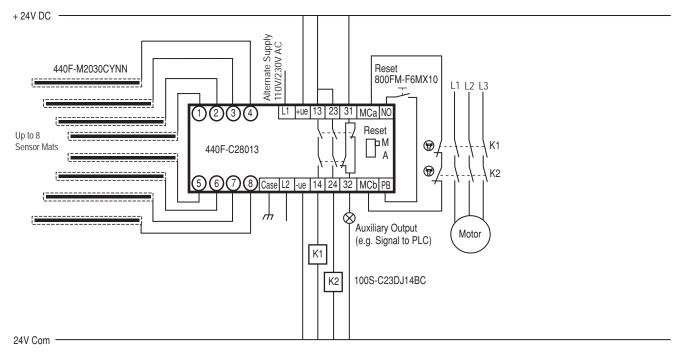
There is no presence on the safety mats. The safety outputs of the Mat Manager are de-energized. The motor is off.
