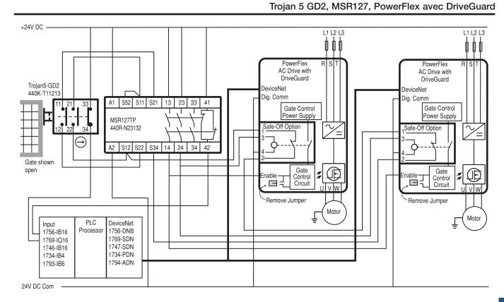
The safety gate is open. The MSR127TP safety outputs (13/14, 23/24, 33/34) are open. The Enable and Safe-Off Option on both PowerFlex drives are off. Auxiliary signals from the Trojan 5 GD2 (33/34) and the MSR127 (41/42) inform the PLC that the safety system is OFF. The motors of both drives are off.
