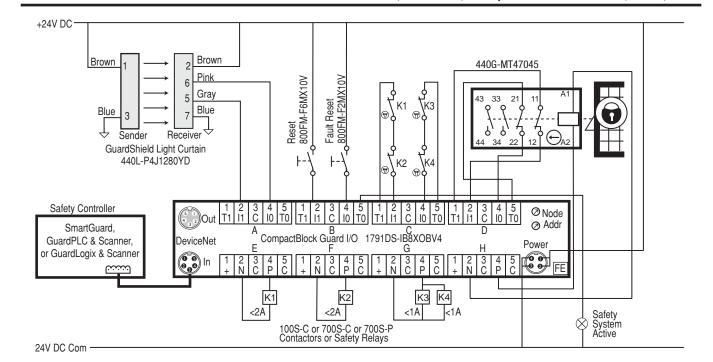
The light curtain is cleared, and the 440G-MT guard locking switch is closed and locked. The contactors K1-K4 are off. The safety system is ready to be energized.
