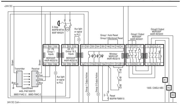
The light curtain is set at the factory default setting (guard only) and is unobstructed. The e-stop is reset. The Group 1 MSR330P safety outputs (13/14, 23/24, 33/34) are on. The Group 3 MSR330P safety outputs are off. K1-K3 are off and ready to be energized.
