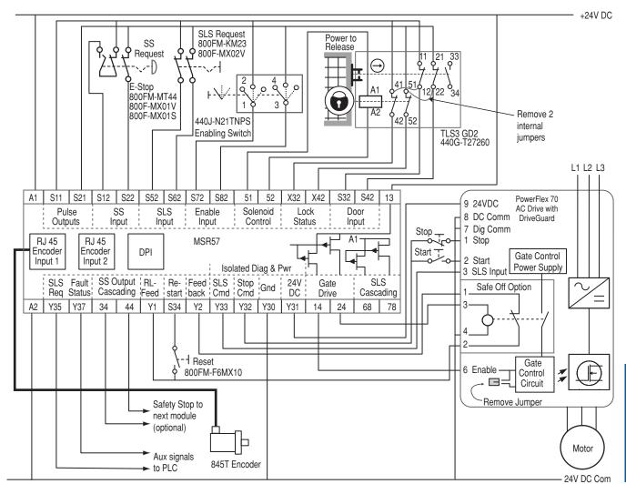
The safe stop (SS) request e-stop button is released. The safe limited speed (SLS) request button is released. The enabling switch is released. The guard locking interlock is closed and locked. The safety outputs (Gate Drive) of the MSR57 are off. The motor is off.
