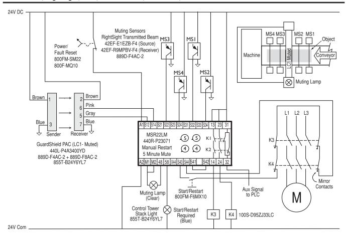
The light curtain is cleared. The muting sensors are cleared. The outputs of the safety relay are de-energized, and the motor is off.
