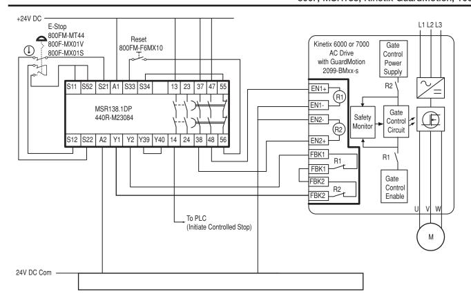
The e-stop is reset. The outputs of the safety relay are open, and the motor is off.
