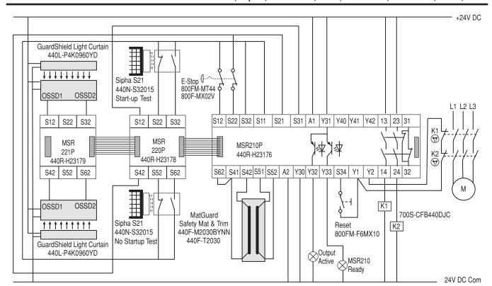
The light curtains are unobstructed. The safety gates are closed. The e-stop is reset and the safety mat is unoccupied. The MSR210 outputs are off. The motor is ready to
