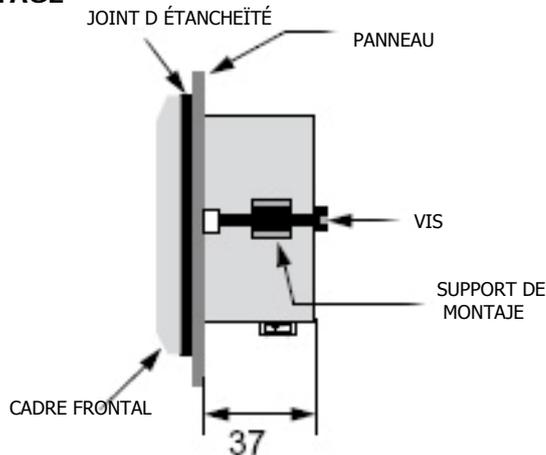
ORIFICE DE MONTAGE: 77 X 163 mm ±0.5 mm
