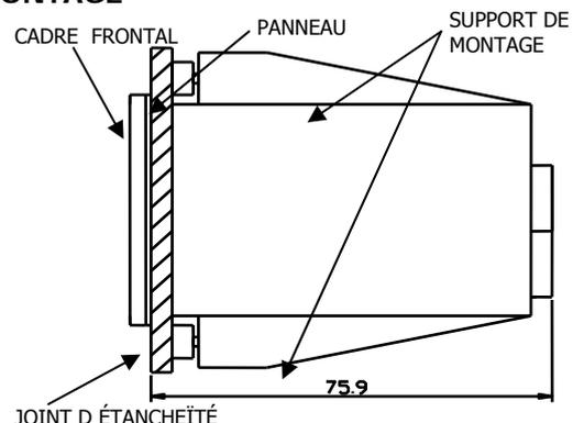
ORIFICE DE MONTAGE: 45 X 45 mm ±0.5 mm
