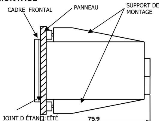
ORIFICE DE MONTAGE: 45 X 45 mm ±0.5 mm
