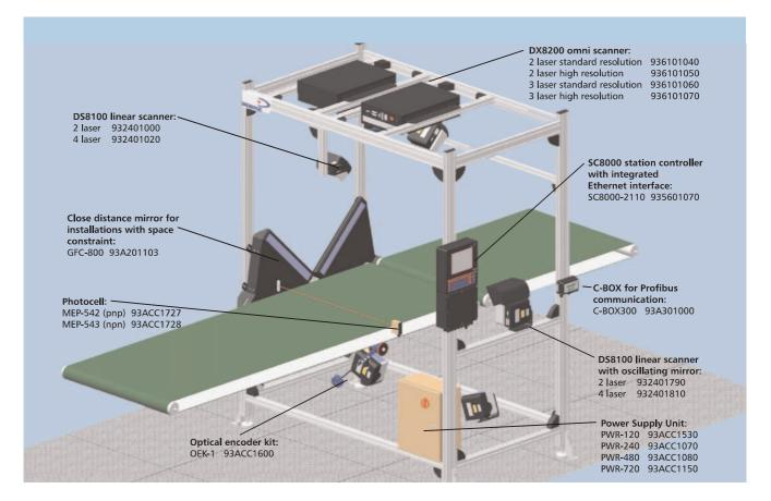
The omni-directional reading station's design includes some standard and particular use accessories. The standard accessories are usually installed and are designed to improve the solution's performance. These accessories include:
