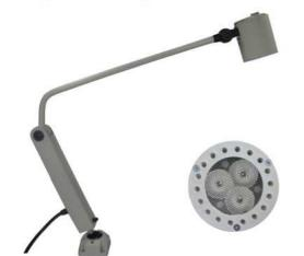
Metal arm lighting system made up of aluminum illuminator covered by anti-heat ABS case with switch on-off, 3 LED sources with 8°-25°-40° lens, head swivel turning, anodized aluminum arm with LED driver, strong aluminum base with sphere and holes for lamp fastening. Power supply 230V 50/60Hz. Current 350mA.
