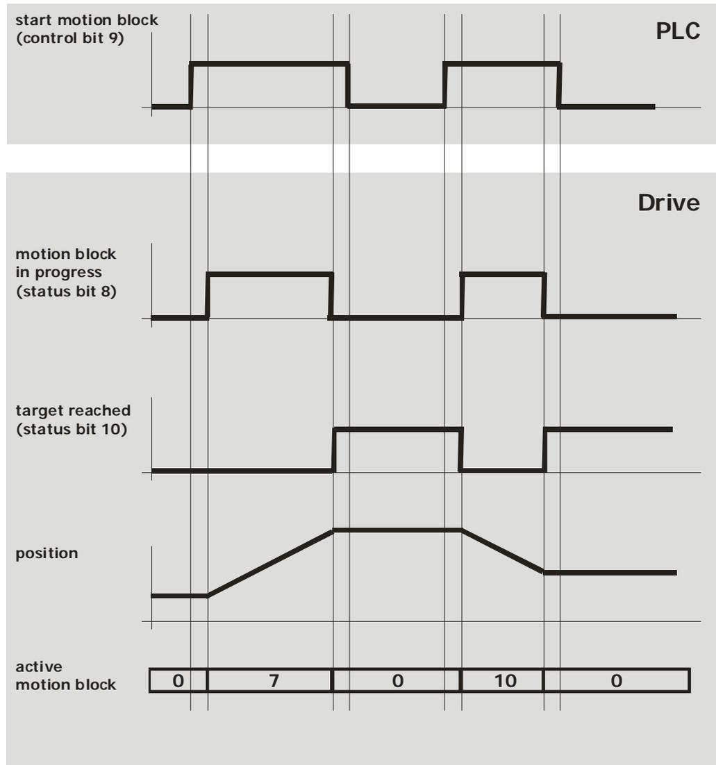
“ motion block sequence” sequence mode (control bit 4) = 1
