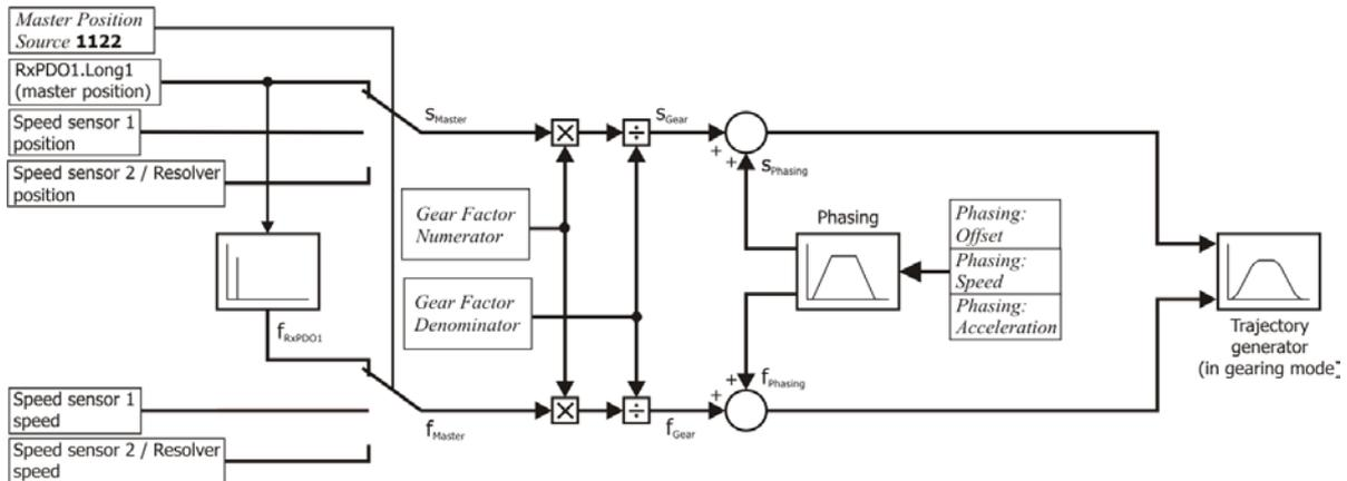
The master position and speed are multiplied by the *gear factor*. When phasing is started, the phasing profile is added to the master speed until the phasing offset is reached.
