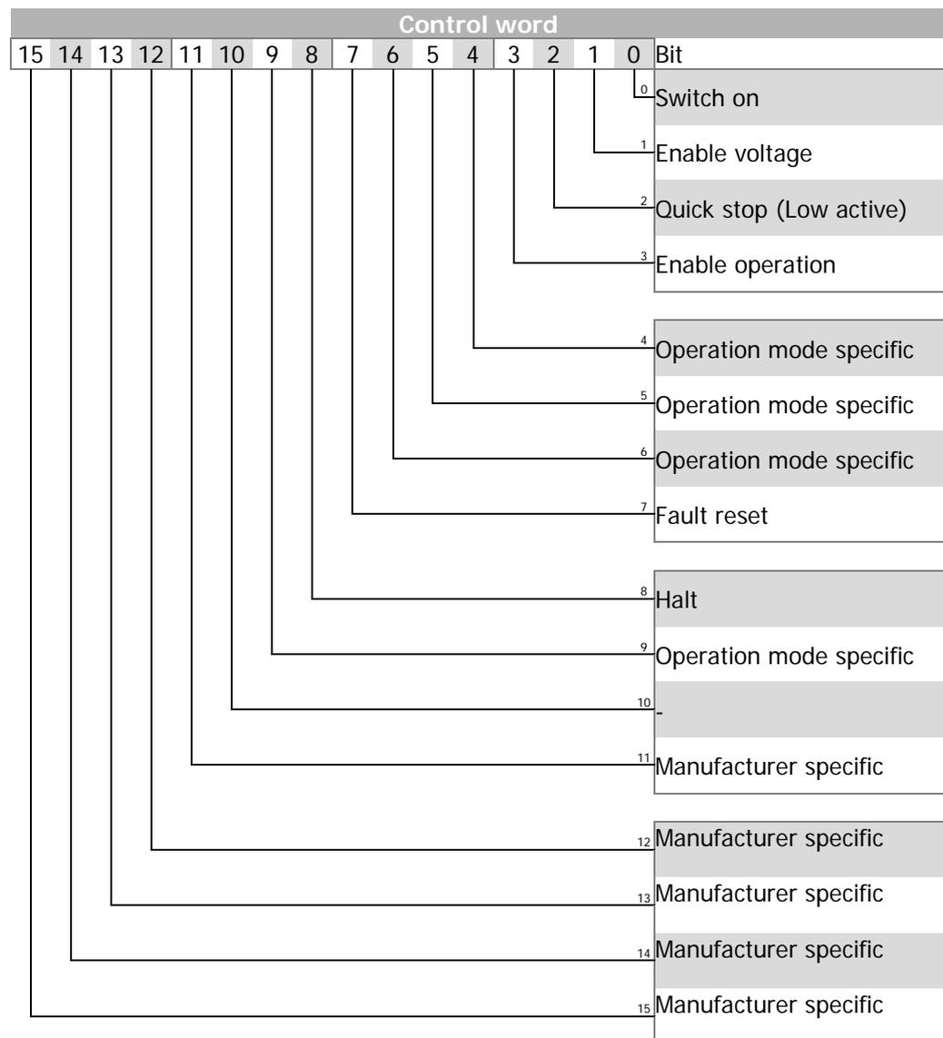
Bits 9 ... 15 are used depending on the configuration and on *Mode of Operation*.
