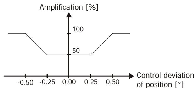
The following behavior may indicate that the controller parameters are not configured properly:
