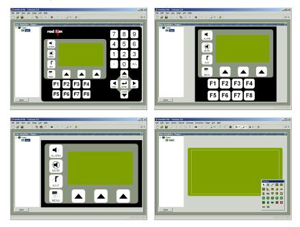
As you can see, at each level, fewer keys are shown, and more of the window is allocated to the display itself. The zoom level can be controlled from the View menu, by using the magnifying glass icon, or by pressing the **Alt** key together with the digits **1** through **4**.
