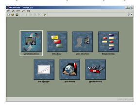
The software is designed such that the first three icons are the only ones required for the majority of simple applications. The remainder of the icons provide access to the terminal's more advanced features, such as programming, data logging and the G3's web server.
