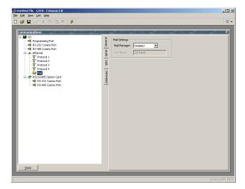
The properties on a General tab are used to enable or disable mail manager, and to provide a name for the operator panel. This name will be used within email messages to identify the originator of the message. Applications will typically use the name of the machine to which the G3 is attached, or the name of the site that it is monitoring.
