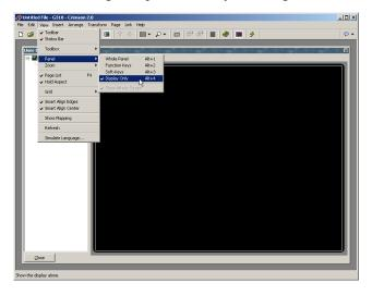
Click on the black screen so the Drawing toolbox appears. To insert the tags on the screen simply click the tag icon <a>[]</a> in the drawing toolbox. In the Select Tag dialog box, select one of the tags and click ok.
