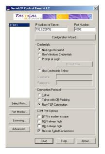
You will now be able to configure any Windows-based software to use the newly-created COM port for download. When the software opens the connection, the G3 will suspend communications on the shared port, and then data will be exchanged between the PC software and the remote PLC—just as if they were connected directly! When the port is closed, or if no data is transferred for a minute, communications will be resumed.
