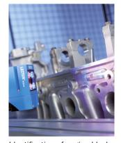
Identification of engine blocks for individual production control and traceability
