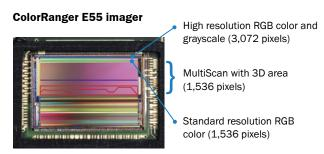
In MultiScan, different parts of the sensor are assigned to different measurement components by software configuration.
