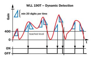
Setting/resetting of switching out-put (only) depending on steep positive/negative edge of an object during trigger time (detecting of edges of objects).
