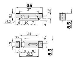
**Cutter FC\* for fibre-optic cables**
