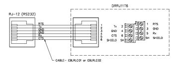
A Red Lion Controls device with an RS232 RJ-12 port is connected to the DRRJ11T6 adapter using the CBLRLC01 or CBLRLC02 cable. The terminal block is then wired to run the RS232 serial information to another device.
